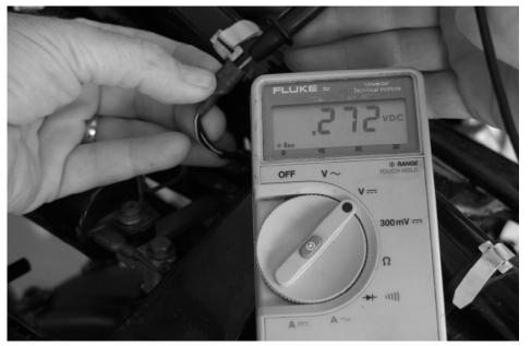
The voltage drop test can uncover resistances too small for an ohmmeter to measure.
